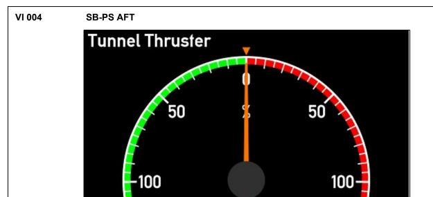
Description: RPM/%RPM SB-PS AFT
